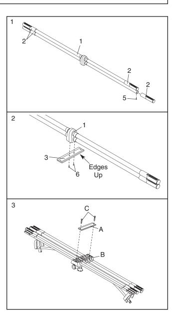
4. Attach the Cover Plate (3) to the Tray (B) with the two Button Head Screws (C) that were removed in step 3. Note: Make sure the decal is over the indicated resistance bars
