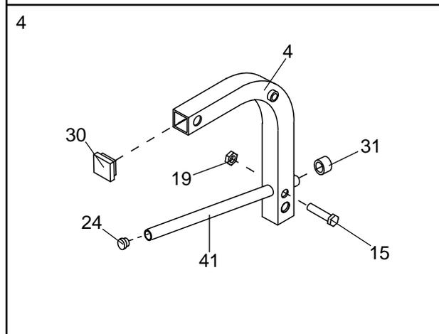
5. Lubricate the 3/8” x 2 1/4” Bolt (14). Attach the Leg Lever (4) to the Main Frame (2) with the 3/8” x 2 1/4” Bolt and a 3/8” Jam Nut (18). Do not overtighten the Jam Nut. The Leg Lever must be able to pivot freely.
