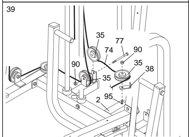
40. Lay the Ab Cable (74) inside the indicated bracket on the Center Base (2). Attach a 90mm Pulley (35) inside the bracket with an M10 x 45mm Bolt (94) and an M10 Nylon Locknut (90).
