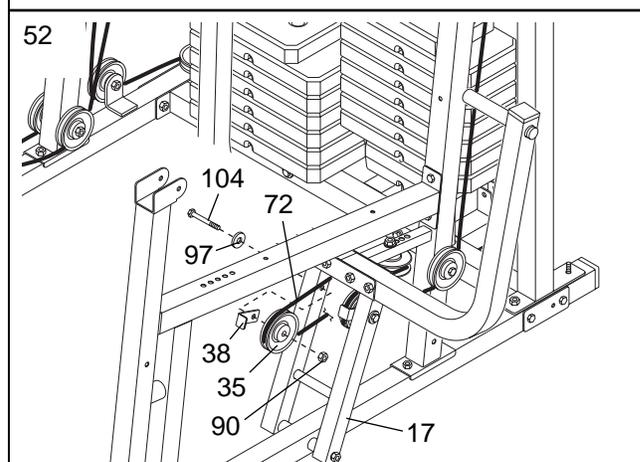
53. Wrap the Press Cable (72) around a 90mm Pulley (35) in the direction shown. Attach the Pulley and a Cable Trap (38) to the indicated hole **on the right side** of the Press Upright (5) with an M10 x 121mm Bolt (102) and an M10 Nylon Locknut (90). **Note: Thread the Locknut only two turns onto the Bolt; another Pulley will be attached to the Bolt in step 57. Make sure the Cable Trap is positioned to hold the Cable in the groove of the Pulley.**
