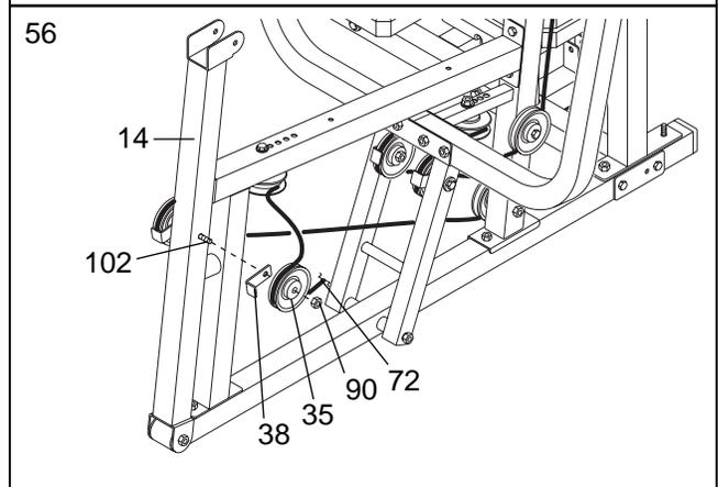
57. Remove the M10 Nylon Locknut (90) used in step 53.
