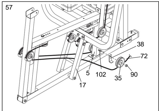
58. Wrap the Press Cable (72) around a 90mm Pulley (35) as shown. Slide a Cable Trap (38) and the Pulley onto the M10 x 92mm Carriage Bolt (112) in the Press Base (3). Secure the Pulley with an M10 Nylon Locknut (90). **Make sure the Cable Trap is positioned to hold the Cable in the groove of the Pulley.**
