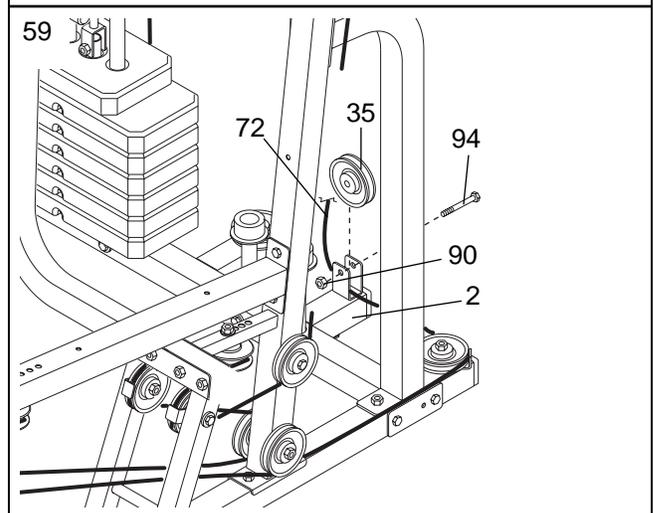
60. Wrap the Press Cable (72) over a 115mm Pulley (36). Attach the Pulley inside the indicated bracket on the Center Top Frame (8) with an M10 x 45mm Bolt (94) and an M10 Nylon Locknut (90).
