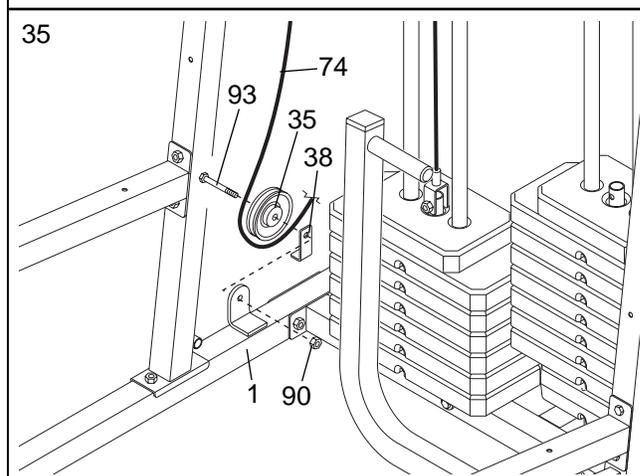
36. Wrap the Ab Cable (74) around a 90mm Pulley (35) in the direction shown. Slide a Cable Trap (38) and the Pulley onto the M10 x 89mm Carriage Bolt (95) in the Butterfly Base (1). Secure the Pulley with an M10 Nylon Locknut (90). **Make sure the Cable Trap is positioned to hold the Cable in the groove of the Pulley.**
