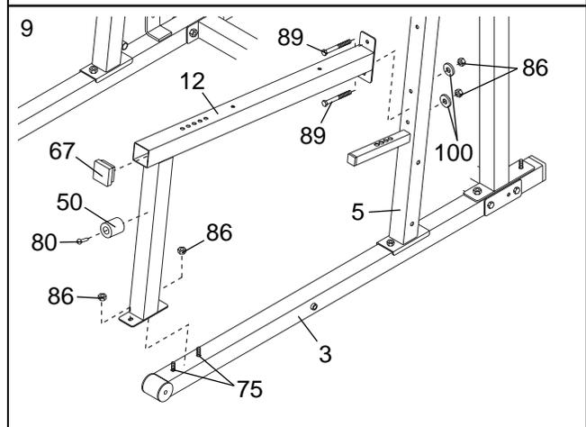
10. Press a 50mm Square Inner Cap (67) into the Press Top Frame (9).
