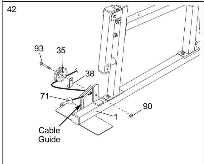
43. Wrap the Low Cable (71) under a 90mm Pulley (35). Attach the Pulley and a Cable Trap (38) to the welded tube on the Butterfly Upright (4) with an M10 x 121mm Bolt (102) and an M10 Nylon Locknut (90). **Note: Thread the Locknut only two turns onto the Bolt, another Pulley will be attached to the Bolt in step 45. Make sure the Cable Trap is positioned to hold the Cable in the groove of the Pulley.**
