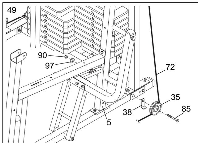
50. Route the Press Cable (72) through the opening in the Press Frame (17) and wrap the Cable around a 90mm Pulley (35) in the direction shown.
