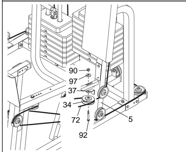
**If a cable slips off the pulleys often, the cable may have become twisted. Remove the cable and re-install it. If the cables need to be replaced, see ORDERING REPLACEMENT PARTS on the back cover of this manual.**
