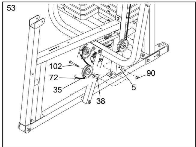
54. Route the Press Cable (72) through the Press Frame (17) and around a 90mm Pulley (35) as shown. Attach the Pulley and a Cable Trap (38) to the indicated hole **on the right side** of the Leg Press Lever (14) with an M10 x 121mm Bolt (102) and an M10 Nylon Locknut (90). **Note: Thread the Locknut only two turns onto the Bolt; another Pulley will be attached to the Bolt in step 56. Make sure the Cable Trap is positioned to hold the Cable in the groove of the Pulley.**
