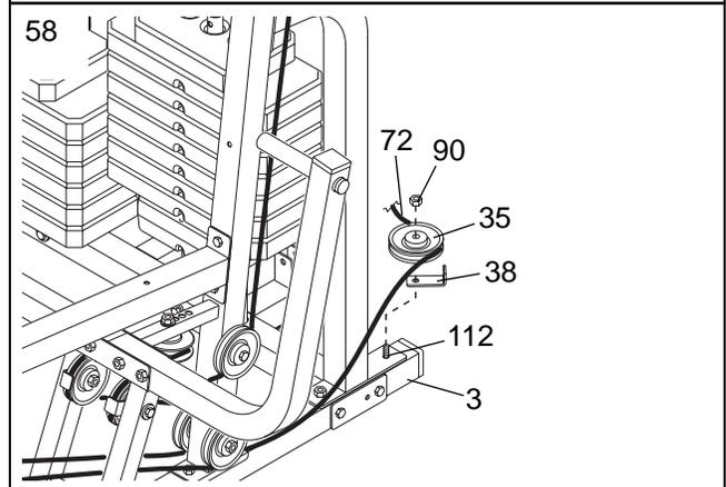
59. Lay the Press Cable (72) in the bracket on the Center Base (2). Attach a 90mm Pulley (35) inside the bracket with an M10 x 45mm Bolt (94) and an M10 Nylon Locknut (90).
