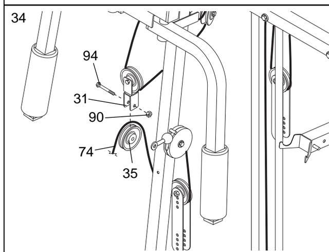
35. Wrap the Ab Cable (74) under a 90mm Pulley (35). Attach the Pulley and a Cable Trap (38) to the indicated bracket on the Butterfly Base (1) with an M10 x 48mm Bolt (93) and an M10 Nylon Locknut (90). **Make sure the Cable Trap is positioned to hold the Cable in the groove of the Pulley.**
