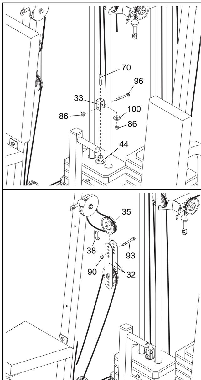
Slack can be removed from the Press Cable (72) by moving the “V”-pulley (34) attached to the Press Seat Frame (12) closer to the Press Upright (5).
