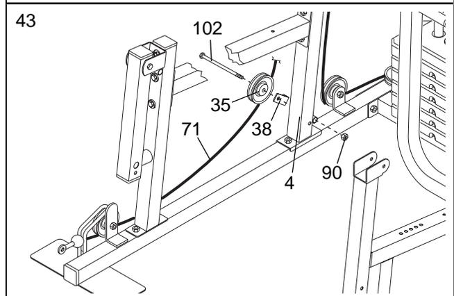
44. Wrap the Low Cable (71) over a 90mm Pulley (35). Attach the Pulley and a Cable Trap (38) to the second set of holes from the bottom in the Pulley Plates (32) with an M10 x 48mm Bolt (93) and an M10 Nylon Locknut (90). **Make sure the Cable Trap is positioned to hold the Cable in the groove of the Pulley.**
