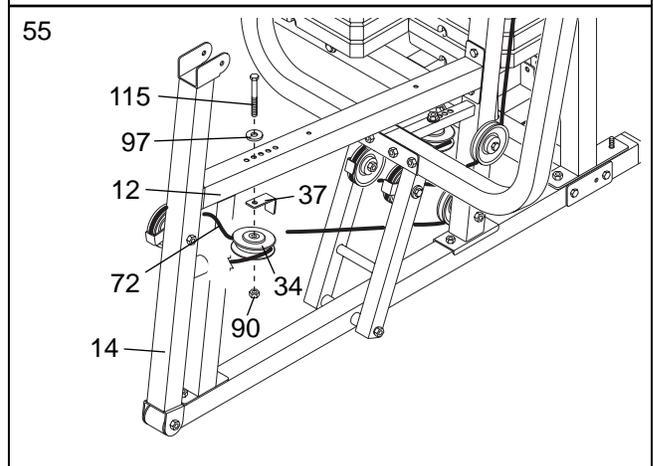
56. **Remove the M10 Nylon Locknut (90) used in step 54.**
