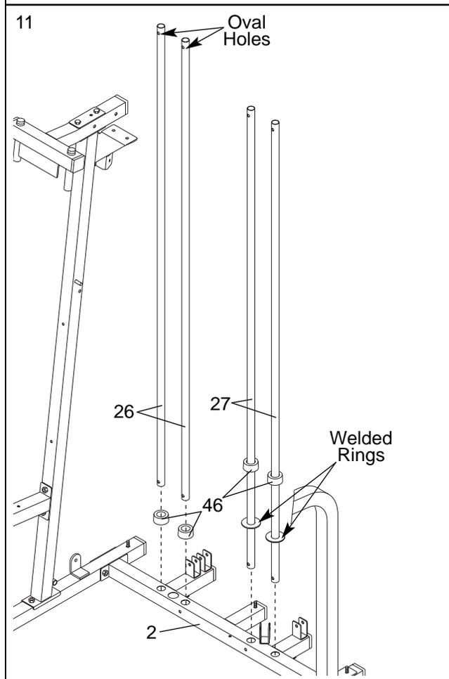
12. Attach the indicated Weight Guides (26, 27) to the Center Base (2) with two M10 x 67mm Bolts (82), four M10 Washers (97), and two M10 Nylon Locknuts (90).
