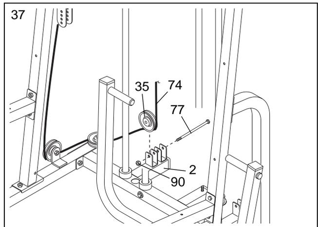
38. Wrap the Ab Cable (74) over a 90mm Pulley (35) in the direction shown. Attach the Pulley and a Cable Trap (38) to the second set of holes from the bottom in the indicated pair of Pulley Plates (32) with an M10 x 48mm Bolt (93) and an M10 Nylon Locknut (90). **Make sure the Cable Trap is positioned to hold the Cable in the groove of the Pulley.**
