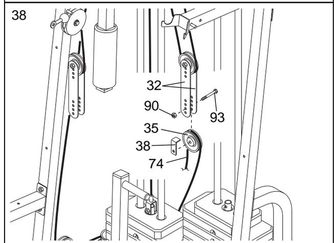
39. **Remove the M10 x 97mm Bolt (77) and the M10 Nylon Locknut (90) used in step 37.**
