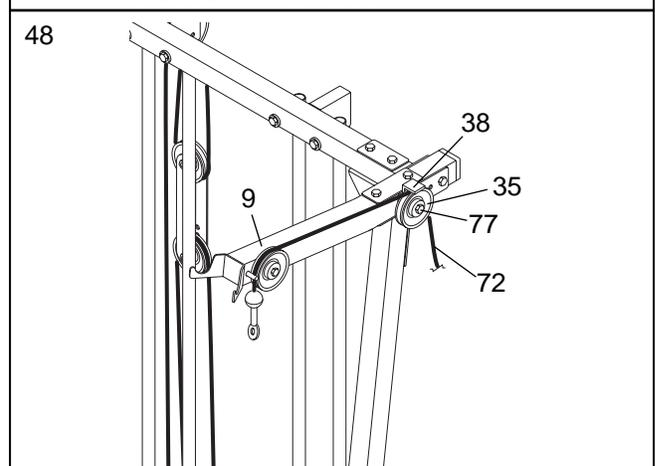
49. Wrap the Press Cable (72) under a 90mm Pulley (35). Attach the Pulley and a Cable Trap (38) to the indicated hole in the Press Upright (5) with an M10 x 93mm Bolt (85), an M10 Washer (97) and an M10 Nylon Locknut (90). **Make sure the Cable Trap is positioned to hold the Cable in the groove of the Pulley.**
