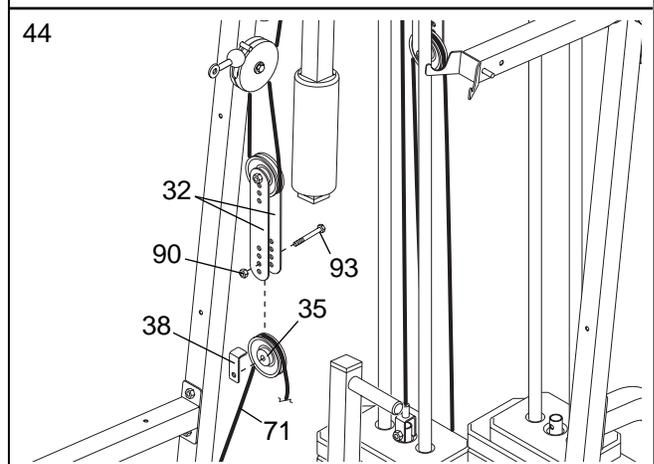
45. Remove the M10 Nylon Locknut (90) used in step 43.
