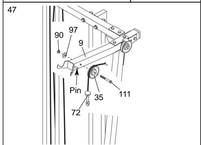
48. Route the Press Cable (72) over the 90mm Pulley (35) that was attached to the Press Top Frame (9) in step 16. **Make sure the Cable Trap (38) is positioned to hold the Cable in the groove of the Pulley.** Properly tighten the M10 Nylon Locknut (not shown) attached to the M10 x 97mm Bolt (77).
