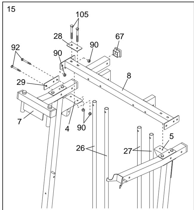
16. Attach the the rear hole in Center Top Frame (8) to the Press Top Frame (9) with an M10 x 69mm Bolt (92), a Large Support Plate (29), and an M10 Nylon Locknut (90). **Do not tighten the Locknut yet.**
