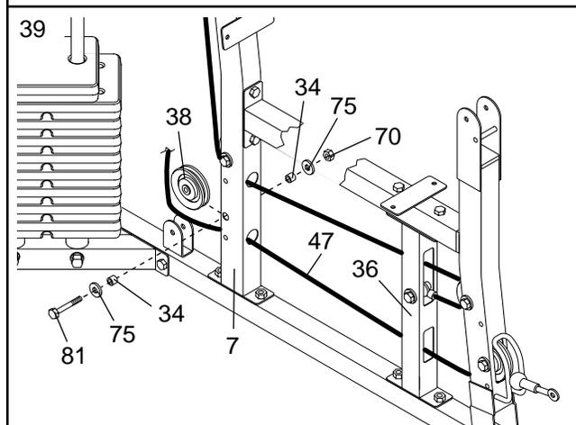
40. Wrap the Low Cable (47) around a 90mm Pulley (38). Attach the Pulley and a Cable Trap (91) to the lower set of holes in the indicated "U"-Bracket (85) with an M10 x 50mm Bolt (62) and an M10 Nylon Locknut (70). **Be sure the Cable Trap is turned to hold the Cable in the groove of the Pulley.**
