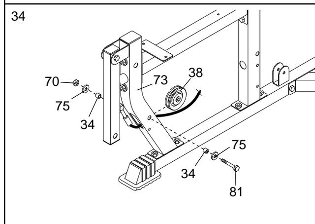
35. Route the Leg Lever Cable (96) through the Right Upright (6) and around a 90mm Pulley (38). Attach the Pulley inside the Upright with an M10 x 70mm Bolt (81), two M10 Washers (75), two 13mm Spacers (34), and an M10 Nylon Locknut (70).
