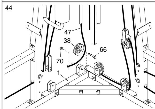
45. Wrap the Low Cable (47) around a 90mm Pulley (38). Attach the Pulley to the indicated bracket on the Right Base (1) with an M10 x 45mm Bolt (66) and an M10 Nylon Locknut (70).
