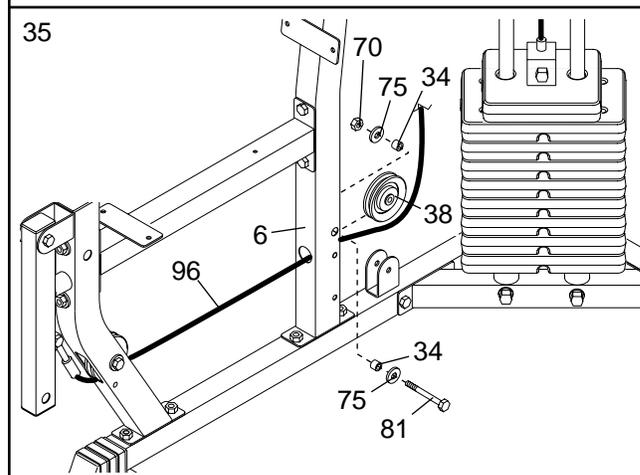
36. Wrap the Leg Lever Cable (96) around a 90mm Pulley (38). Attach the Pulley and a Cable Trap (91) to the second set of holes from the bottom of the indicated Double "U"-Bracket (56) with an M10 x 50mm Bolt (62) and an M10 Nylon Locknut (70). **Be sure the Cable Trap is turned to hold the Cable in the groove of the Pulley.**
