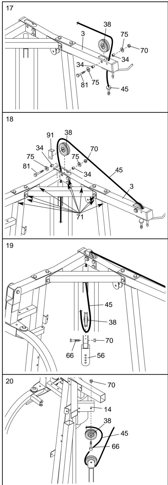
21. Wrap the High Cable (45) around a 90mm Pulley (38). Attach the Pulley at the forward hole, inside the bracket on the Center Top Frame (14) with an M10 x 45mm Bolt (66) and an M10 Nylon Locknut (70).
