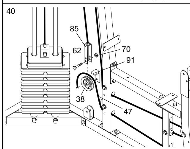
41. Wrap the Low Cable (47) around a 90mm Pulley (38). Attach the Pulley to the indicated bracket on the Left Base (2) with an M10 x 45mm Bolt (66) and an M10 Nylon Locknut (70).
