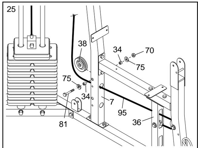
26. Wrap the Leg Press Cable (95) around a 90mm Pulley (38). Attach the Pulley inside the bracket on the Left Top Frame (3) with an M10 x 45mm Bolt (66) and an M10 Nylon Locknut (70).
