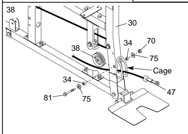
39. Route the Low Cable (47) through the Left Leg (36) and the Left Upright (7). Attach a 90mm Pulley (38) inside the Upright with an M10 x 70mm Bolt (81), two M10 Washers (75), two 13mm Spacers (34), and an M10 Nylon Locknut (70).
