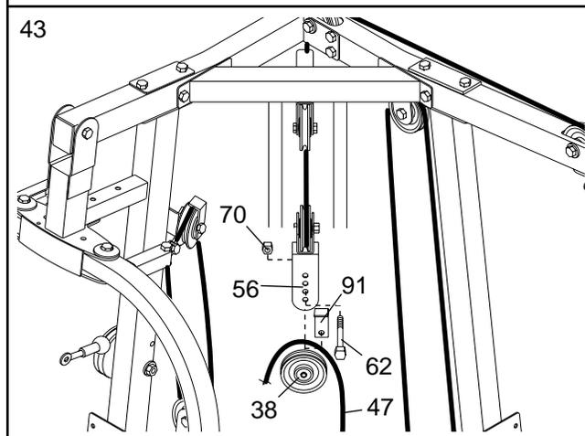
44. Wrap the Low Cable (47) around a 90mm Pulley (38). Attach the Pulley to the indicated bracket on the Right Base (1) with an M10 x 45mm Bolt (66) and an M10 Nylon Locknut (70).
