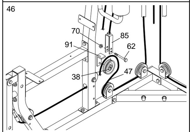
47. Wrap the Low Cable (47) around a 90mm Pulley (38). Attach the Pulley and a Cable Trap (91) to the side of the Right Upright (6) with an M10 x 95mm Bolt (98), an M10 Washer (75), and an M10 Nylon Locknut (70). **Be sure the Cable Trap is turned to hold the Cable in the groove of the Pulley.**
