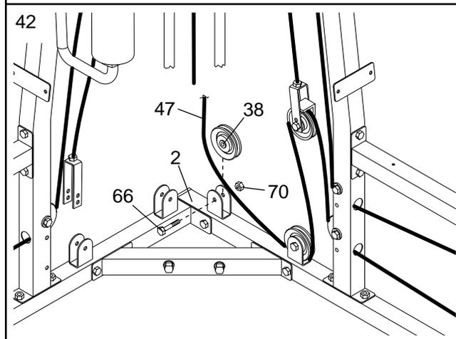
43. Wrap the Low Cable (47) around a 90mm Pulley (38). Attach the Pulley and a Cable Trap (91) to the second set of holes from the bottom of the indicated Double "U"-Bracket (56) with an M10 x 50mm Bolt (62) and an M10 Nylon Locknut (70). **Be sure the Cable Trap is turned to hold the Cable in the groove of the Pulley.**
