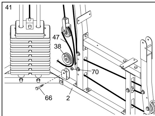
42. Wrap the Low Cable (47) around a 90mm Pulley (38). Attach the Pulley to the indicated bracket on the Left Base (2) with an M10 x 45mm Bolt (66) and an M10 Nylon Locknut (70).
