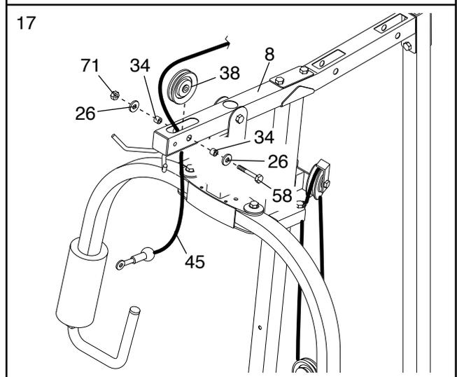
18. Wrap the High Cable (45) around a 90mm Pulley (38). Attach the Pulley inside the Top Frame (8) with an M10 x 70mm Bolt (58), two M10 Washers (26), two 13mm Spacers (34), and an M10 Nylon Locknut (71).
