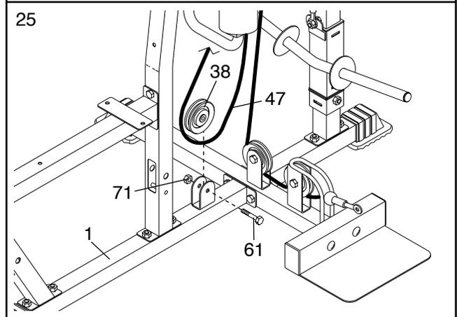
26. Wrap the Low Cable (47) around a 90mm Pulley (38). Attach the Pulley to the Double “U”-Bracket (37) with an M10 x 47mm Bolt (61) and an M10 Nylon Locknut (71).
