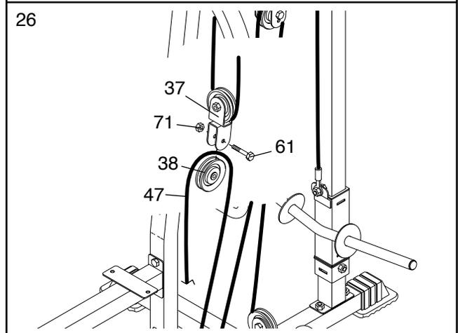
27. Wrap the Low Cable (47) around a 90mm Pulley (38). Attach the Pulley inside the Front Upright (6) with an M10 x 70mm Bolt (58), two M10 Washers (26), two 13mm Spacer (34), and an M10 Nylon Locknut (71).
