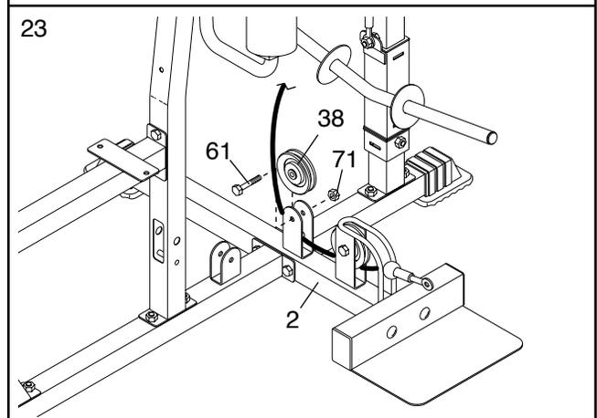
24. Wrap the Low Cable (47) around a 90mm Pulley (38). Attach the Pulley and a Cable Trap (44) to the second set of holes from the bottom of the two Pulley Plates (36) with an M10 x 47mm Bolt (61) and an M10 Nylon Locknut (71). **Be sure the Cable Trap is turned to hold the Cable in the Groove of the Pulley.**
