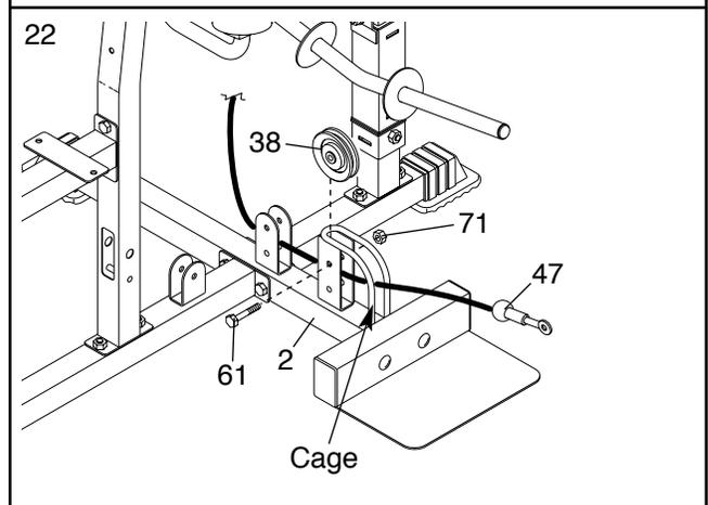
23. Attach a 90mm Pulley (38) inside the indicated bracket on the Center Base (2) with an M10 x 47mm Bolt (61) and an M10 Nylon Locknut (71).
