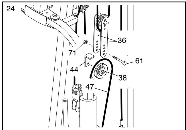
25. Wrap the Low Cable (47) around a 90mm Pulley (38). Attach the Pulley inside the indicated bracket on the Front Base (1) with an M10 x 47mm Bolt (61) and an M10 Nylon Locknut (71).
