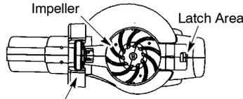
3. Turn the inlet restrictor counterclockwise and remove it from the unit. Do not close the inlet door. You will next attach the vacuum tubes.
