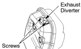
Replace the spark arresting screen every 50 hours of operation or if any damage or breaks in the screen are noted.
