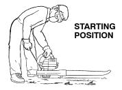
**WARNING:** When starting engine, hold the unit as illustrated. Do not set unit on any surface except a clean, hard area when starting engine or while engine is running. Debris such as gravel, sand, dust, grass, etc. could be picked up by the air intake and thrown out through the discharge opening, damaging the unit or property, or causing serious injury to bystanders or the operator.
