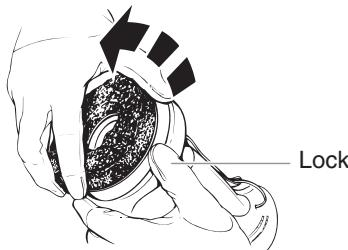
2. While pressing the disc lock on the bottom of the unit, thread new disc onto unit by turning it clockwise and tightening by hand.
