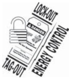
**△WARNING** Always perform the **LOCKOUT / TAGOUT PROCEDURE** before removing any sheet metal panels or attempting to service this equipment. **FAILURE TO COMPLY WITH THIS PROCEDURE CAN CAUSE PROPERTY DAMAGE, INJURY OR DEATH.**
