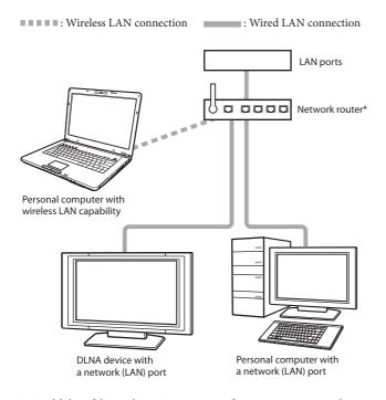
Availability of the wireless LAN access point function on your network router is not relevant in this network topology.
