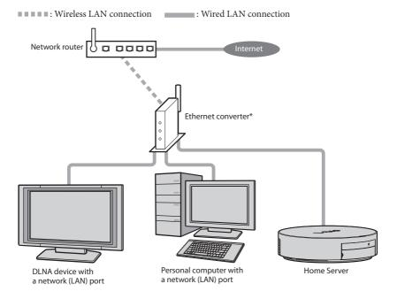
\* The Ethernet converter should have no router or firewall functions.
