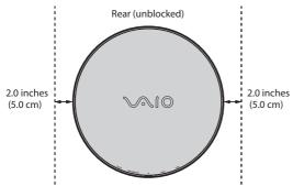
Keep the air-intake vents on the bottom, the sides, and the back of your Home Server unblocked. Place the Home Server on a flat, solid surface so as to let the air flow under the bottom of the Home Server.
