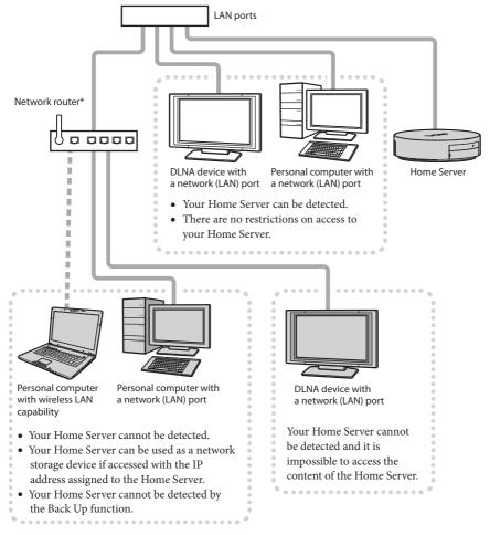
\* If your network router has a bridging function, you can enable the function to eliminate the above restrictions but you may have a problem with the maximum number of connections.
