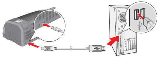
3 Plug the flat end of the cable into any available USB port on your computer.
