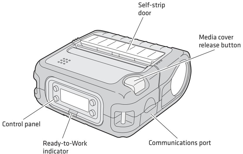
**PB50 Printer:** This illustration shows the important features of the PB50 printer. A weather-resistant flap protects the communications ports and the external power connector.
