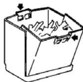
4. Dump compacted trash from half basket into waste receptacle.
