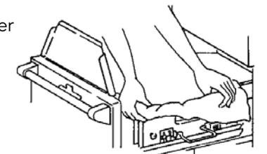
5. Lock bag in place by pulling four pre-punched holes over buttons on drawer sides. Holes will expand over buttons without damaging bag.
