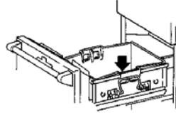
2. Put trash directly into the basket. We recommend placing several thicknesses of newspaper at the bottom of the basket when bags are not used. This will minimize clean-up of the basket after emptying compacted trash.
