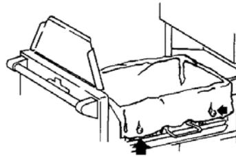
6. Spread bag to fit interior of basket. Closing storage compartment cover. Pull basket release handle up.
