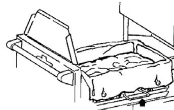
2. Lift storage compartment cover up. Release bag from buttons. Pull up top edges of bag.
