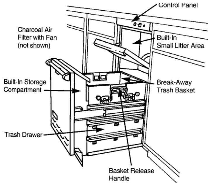
Your compactor has a built-in interlock and will not operate unless you have:
