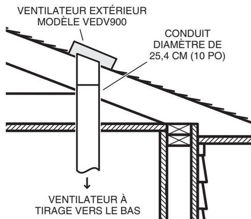
POSE TYPE - VENTILATEUR MONTÉ SUR LE TOIT
