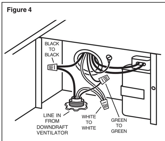
6. Make the electrical connections with the proper connector for the type of wiring being used. Connect white to white, black to black, and the green or bare wire to green. See Figure 4.
