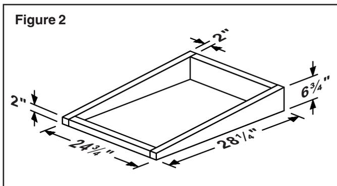
5. For flat roof installations, build a curb that will mount the blower at a minimum pitch of 2/12. See Figure 2. Discharge end of the blower should be pointed away from prevailing winds.
