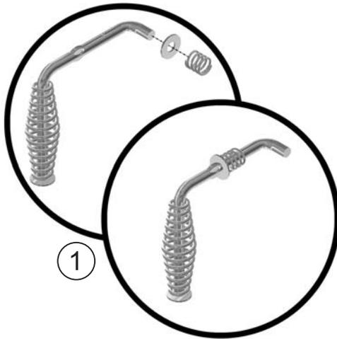
1. Slide the handle washer onto the end of the door handle, followed by the handle spring as shown.
