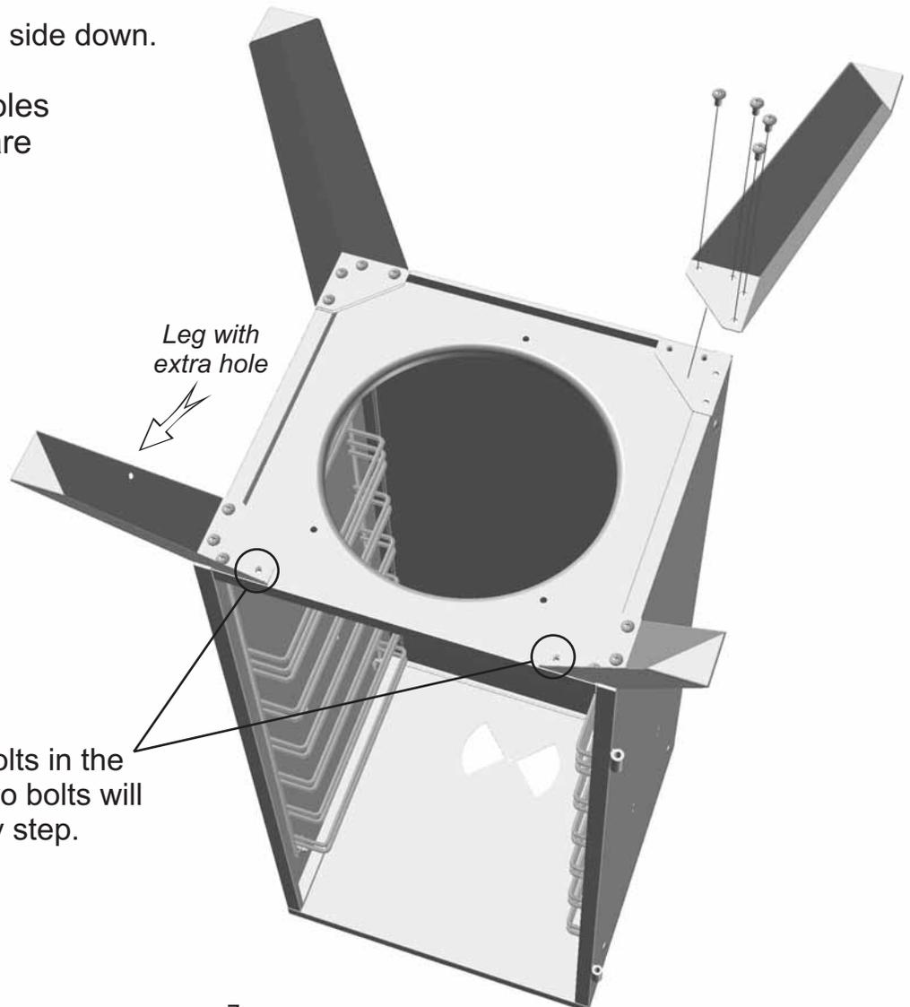
3. DO NOT yet insert the two bolts in the locations indicated. These two bolts will be used in the next assembly step.
