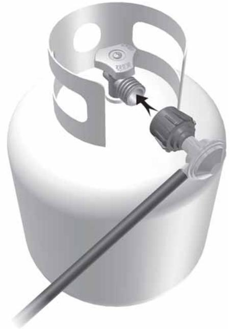
**CAUTION:** In the connection process, the HVR side of the connection will seal on the back check in the valve, resulting in a slight resistance. The connection requires about one-half to three-quarters additional turn to complete the connection.
