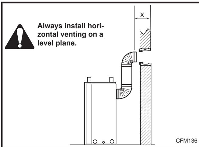
Fig. 27 Measure horizontal length including 2" overlap.
