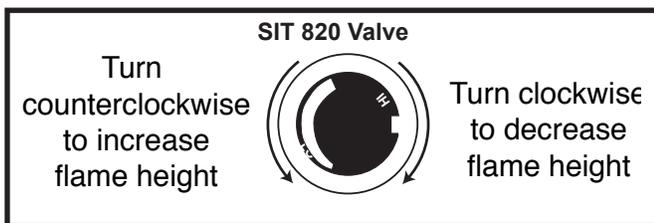
Fig. 59 Flame adjustment knob for SIT valve.
