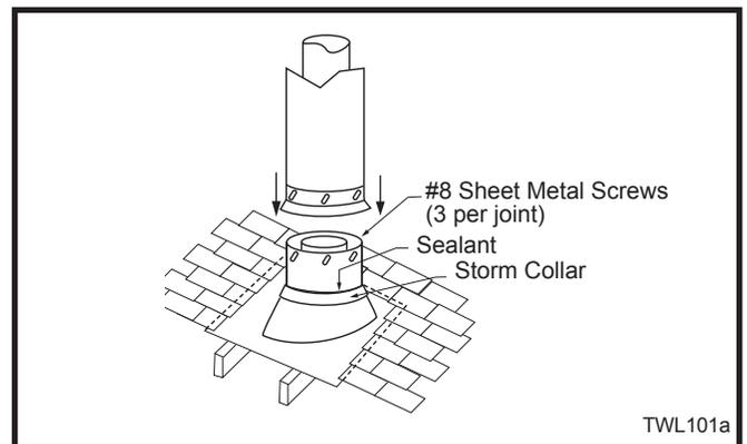
Fig. 54 Roof flashing.
