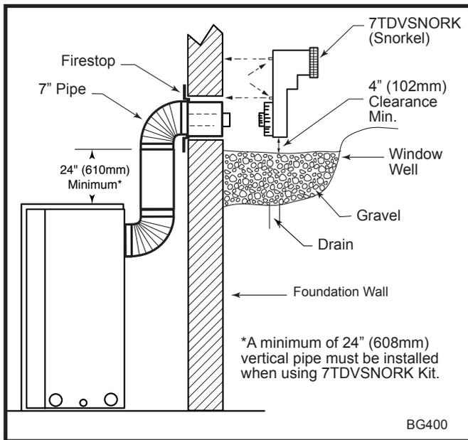
Fig. 30 Below grade installation.
