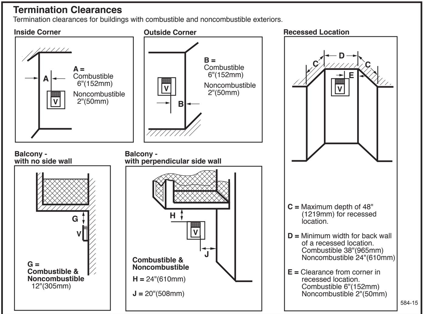
Fig. 8 Termination clearances.
