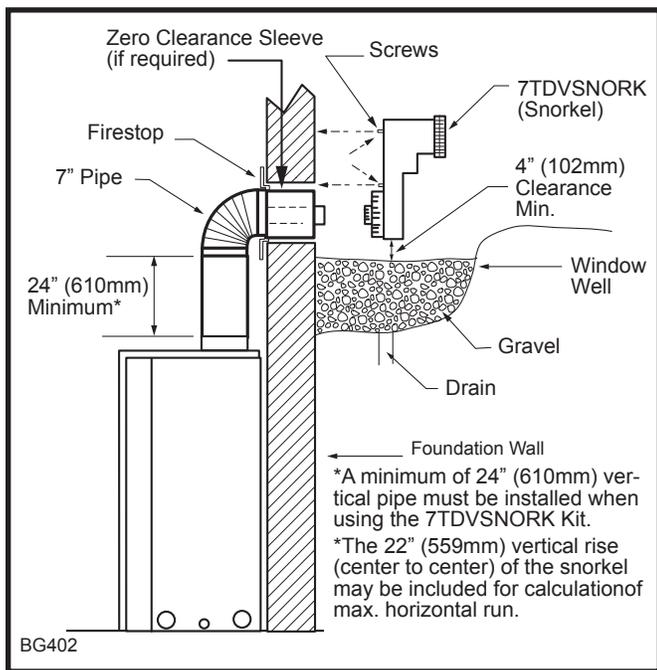
Fig. 48 Below grade installation.
