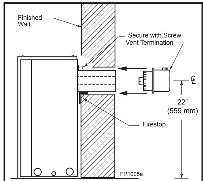
Fig. 15 Side view of final unit location.
