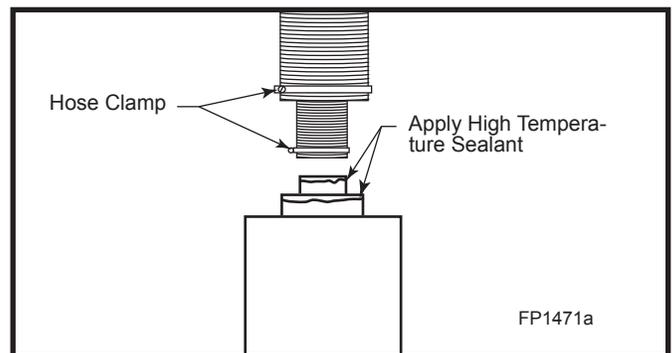
Fig. 9 Apply high temperature sealant to 4" and 7" pipes.
