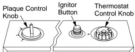
**Figure 23 - Thermostat Control Knob In The OFF Position, Models VP16TA & VN22TA**
