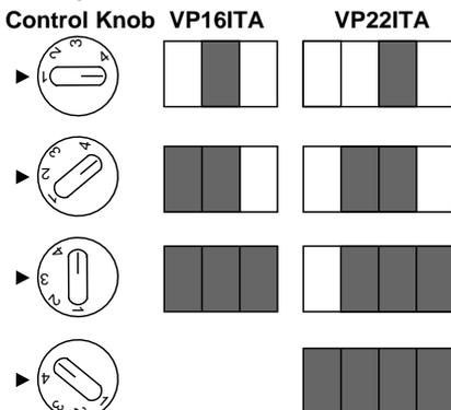
Figure 26 - Burner Patterns, Models
