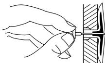
Figure 10 - Popping Open Anchor Wings For Thin Walls
