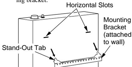
Figure 11 - Mounting Heater Onto Mounting Bracket
