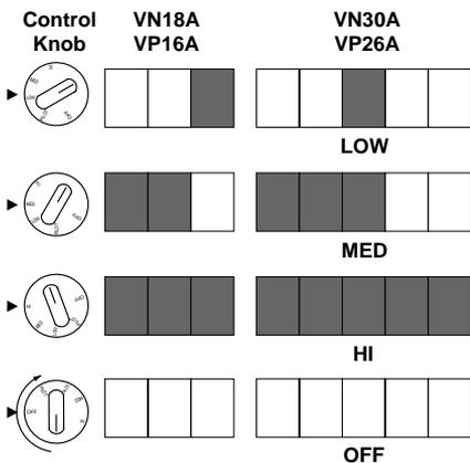
Figure 21 - Burner Patterns for Non-Thermostat Models
