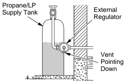
**Figure 14 - External Regulator With Vent Pointing Down**
