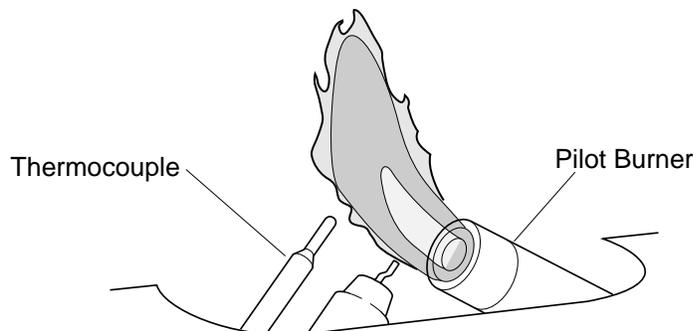
**Figure 24 - Incorrect Pilot Flame Pattern**
