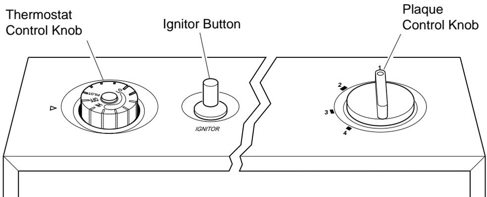
Figure 17 - Thermostat Control Knob In The OFF Position
