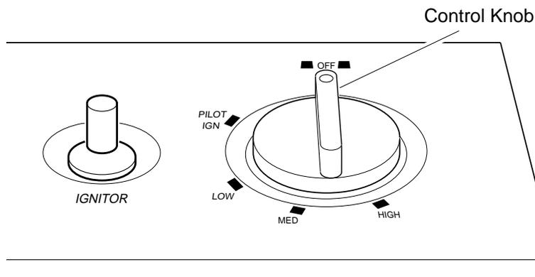
Figure 20 - Control Knob In The OFF Position
