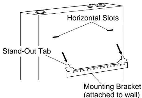
**Figure 11 - Mounting Heater Onto Mounting Bracket**
