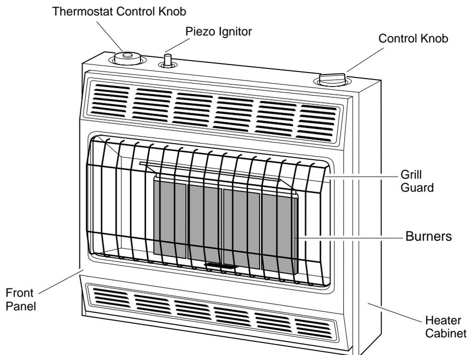
Figure 1 - Vent-Free Natural Gas Heater (Model VN2550ITB Shown)
