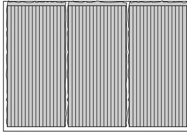
Figure 21 - Correct Burner Flame Pattern
