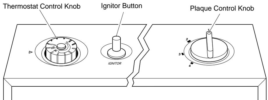
Figure 16 - Thermostat Control Knob In The OFF Position
