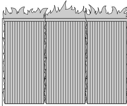
Figure 22 - Incorrect Burner Flame Pattern
