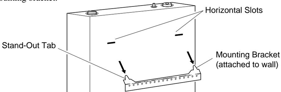
**Figure 10 - Mounting Heater Onto Mounting Bracket**
