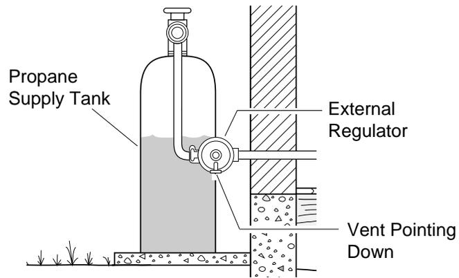
Figure 12 - External Regulator With Vent Pointing Down
