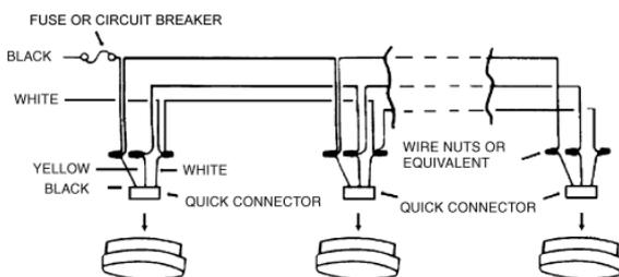
MULTIPLE UNIT INSTALLATION SET-UP
