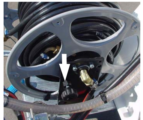
Anti-unwinding blocking knob.
