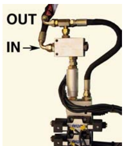
Elettroil connection to quick-fit couplings of the tractor
