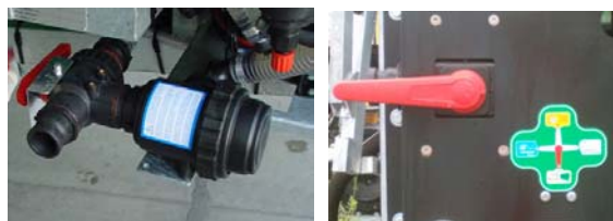
3-way deviator for filling tank
