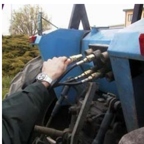
Elettroil connection to quick-fit couplings of the tractor
