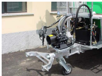
Tractor coupling for Towed machines: standard version, with elevator coupling.
