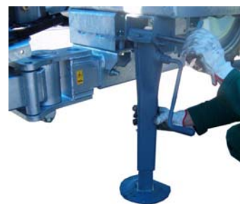
Tractor coupling for Towed machines: homologated version, coupled to tow hook
