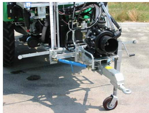
Tractor coupling for Towed machines: homologated version, coupled to tow hook
