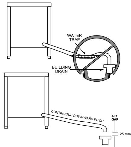
**Leave an air gap between the hose and the building drain, and don't allow water traps in the hose.**
