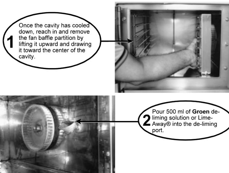
**1** Once the cavity has cooled down, reach in and remove the fan baffle partition by lifting it upward and drawing it toward the center of the cavity.
