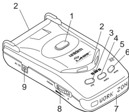
1. **Clip Release** — Press the clip release button to remove the LRD 6699SWS from the windshield mounting clip.
