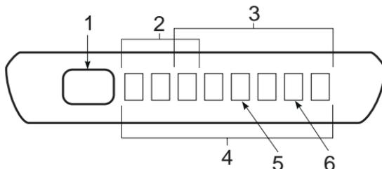
1. **Three-Color LED** — Red indicates a radar detection; Green indicates a laser detection; and Amber indicates a Safety Warning System(SWS) message.
