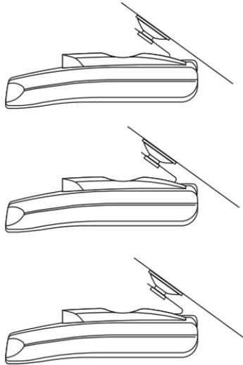
1. The metal portion of the bracket locks into the plastic portion at three different positions. These positions can be used for vehicles with different vertical windshield angles. The back position can be used for vehicles with windshields that are slanted back.
