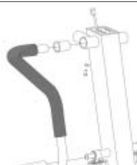
Slide bushing and the upper end of the left handlebar into the mount on the upper end of the vertical frame. Slide the lower end over the spacer. Secure the top of the handlebar with one M8x20 button head bolt and lock washer using the 5 mm hexagon key provided. Attach the right handlebar in the same manner.
