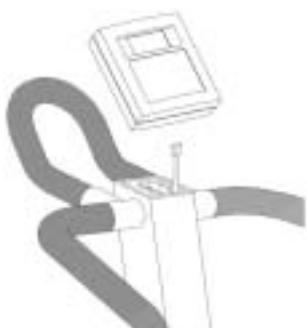
Open the battery case cover on the back of the meter case and insert two 1.5 V AA-batteries to the battery case following the + and - markings. Plug the meter cable into the socket on the rear of the meter. Secure the meter into place by setting it on the meter mount and sliding it down until firmly in place. **NOTE!** Make sure the meter cable is not pinched during the assembly as this can cause the meter to not function correctly.
