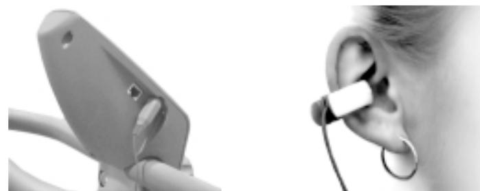
Keep the ear sensor clean. Clean the ear sensor after use with a damp cloth and dry carefully.
