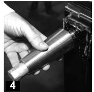
**4** Thread leg into cabinet bottom frame rail.
