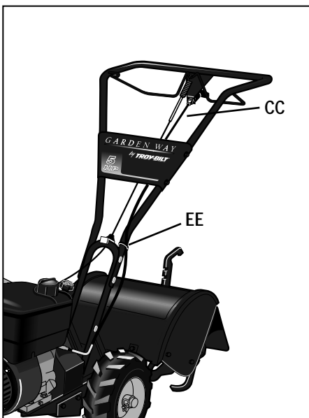
Fig. 2-9: Route reverse clutch cable (CC) as shown. Attach to handlebar with cable tie (EE).
