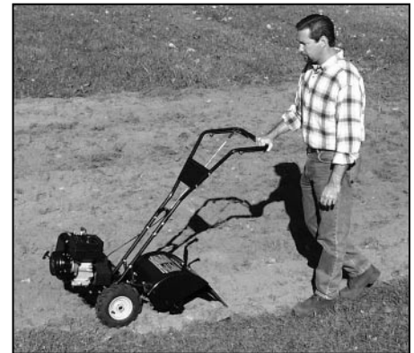
Figure 4-2: Use one hand to guide tiller when moving forward.
