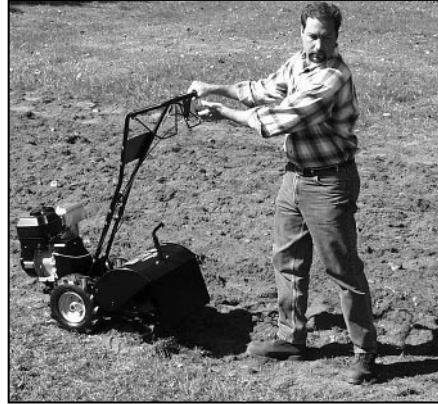
Figure 4-3: Raise tines off ground and look behind when moving in reverse. (Models 12191 and 12193 have powered reverse; Model 12190 can be “fishtailed” backward manually for a short distance, or rolled backward when wheels are in FREEWHEEL.)
