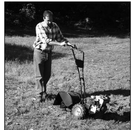
Figure 4-5: With tiller balanced over wheels (and tines out of the ground), push handlebars sideways to turn tiller.
