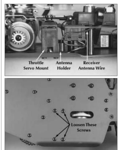
O 2. Uncoil the bundled receiver antenna wire. Run the receiver antenna wire through your fingers to straighten the receiver wire. Thread the antenna wire through the bottom side of the antenna holder which is mounted on the outer throttle servo mount. Loosen, but do not remove the screws in the throttle servo mount.
