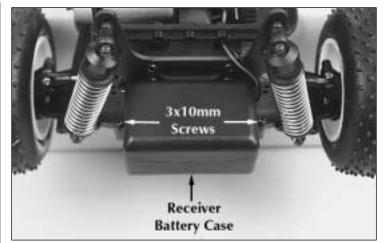
O 5. Remove the two 3x10mm screws from the receiver battery case which is located on the rear of the truck. Then remove the cover from the top of the receiver battery case.
