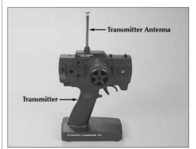
**O** 7. Remove the transmitter antenna from the parts bag and install it into the top of the transmitter as shown. To ensure that the antenna is attached, lightly pull on the antenna. If it slides out, it is not screwed in properly.
