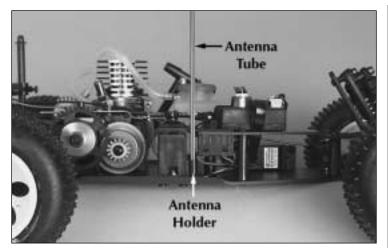
**O** 3. Remove the antenna tube from the parts bag. Run the antenna through your fingers a few more times to straighten the receiver antenna wire. Thread the receiver antenna wire through the antenna tube. Press fit the antenna tube into the antenna holder which is located on the throttle servo mount. **Do not cut or coil the receiver antenna wire**.
