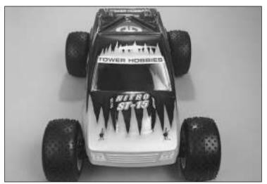
**O** 10. Remove the clear lexan truck body from the box. Prepare the lexan body to be painted by washing it out with warm water and a liquid detergent. Dry the body off with a non-abrasive cloth.
