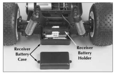
$\bigcirc$  6. Remove the receiver battery holder from the receiver battery case. Install 4 (included) "AA" batteries into the battery holder in the configuration molded into the battery holder. Re-install the battery holder and the battery case top with the two 3x10mm screws which you removed earlier.
