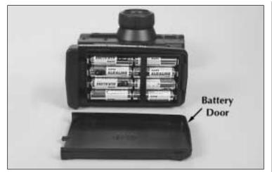
**O** 8. Slide off the battery door on the bottom of the transmitter. Install 8 "AA" batteries into the bottom of the transmitter in the configuration molded into the battery holder. Re-install the battery door onto the bottom of the transmitter.
