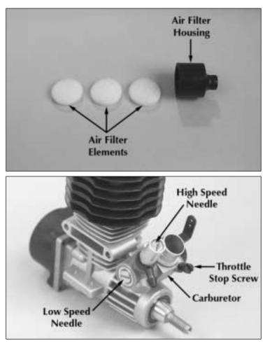
**O** 4. Remove the air filter from the parts bag. Remove the 3 air filter elements from the air filter housing and soak the air filter elements with air filter oil (not included) and then squeeze the excess oil from the elements. A light shock oil may be used or you can purchase special air filter oil from most hobby shops. Place the air filter elements back into the air filter housing, and then install the air filter assembly onto the top of the carburetor.
