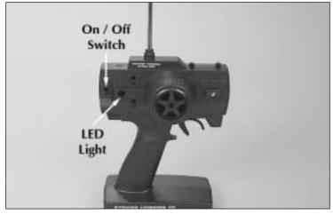
**O** 9. Turn the transmitter on using the switch on the front. The red LED light next to the on/off switch should light up. If the LED does not light up, turn the transmitter off and check to make sure the batteries are properly installed in the bottom of the transmitter. Turn the transmitter on again to make sure the red LED lights, and if it does turn the transmitter off. If the LED light is blinking, the batteries are low and should be replaced!
