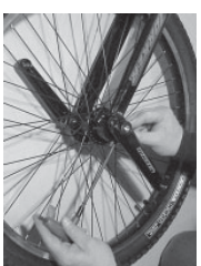
B] Use Hardware bolts to attach Bearing Caps.
