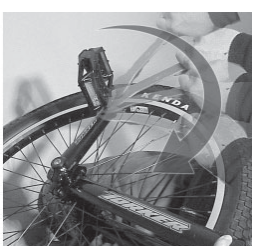
D2] The right pedal tightens clockwise.
