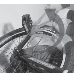
D1] Left pedal tightens counter-clockwise.
