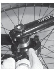
A] Place Wheel in Bearing Cradle and place on Caps.
