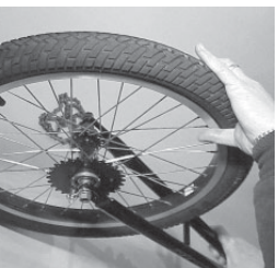
B Place wheel in fork slots loosely.
