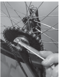
I Tighten chain adjusters to pull chain tight. Be sure to keep wheel centered (below).
