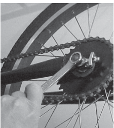
J Now tighten axle nuts. Then, attach correct pedals on to correct crank arms. ** Read directions for specifics.
