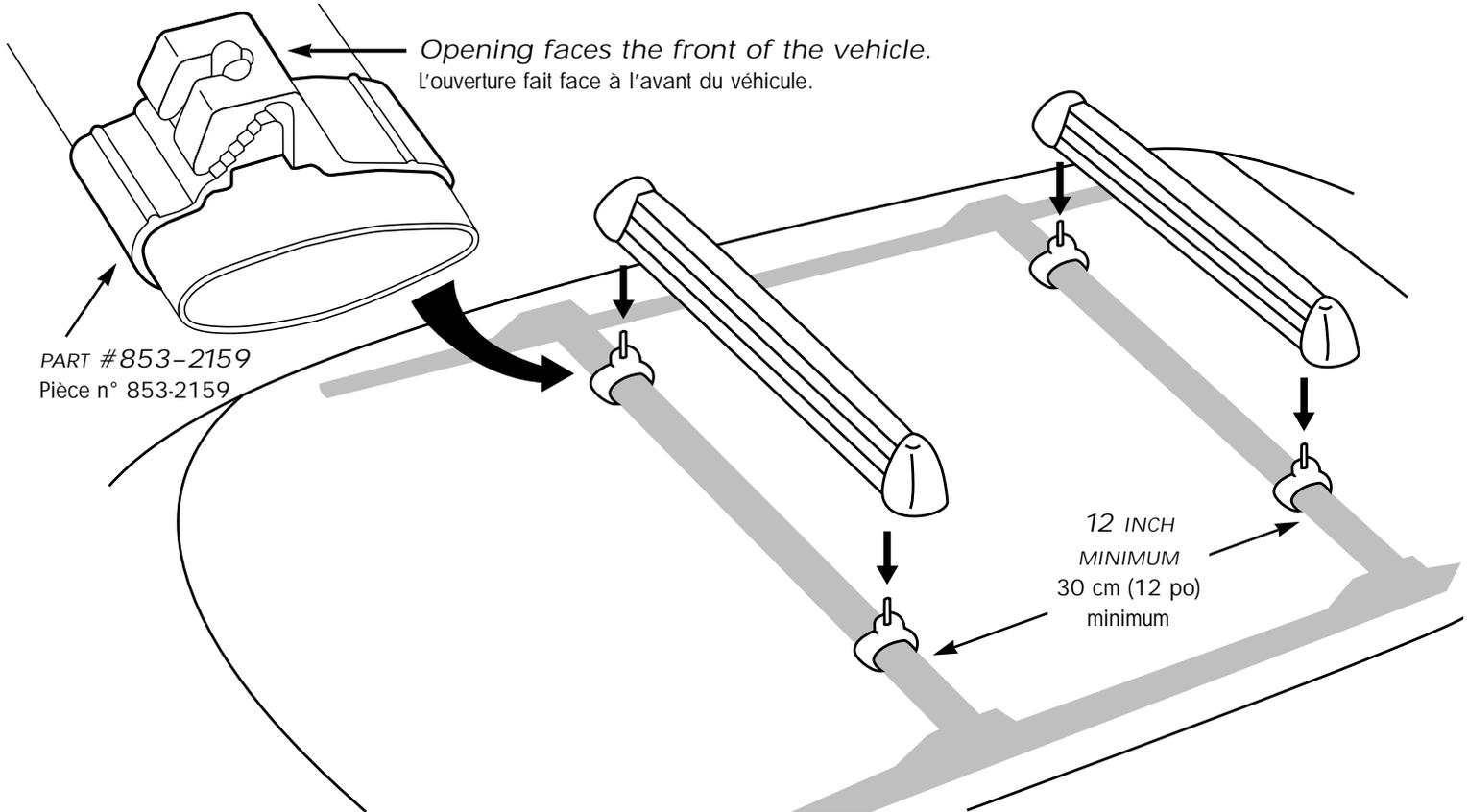
■ Minimum required load bar spread is 12 inches.
