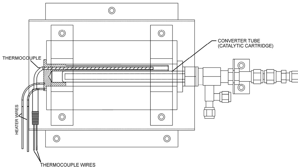
**Figure 4-2. Thermocouple Location**
