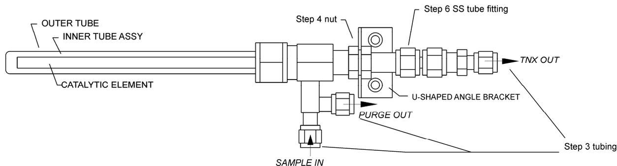
**Figure 4-1. Catalytic Cartridge**
