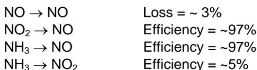
As can be seen from the above reactions, the calculation of the ammonia concentration and overall calibration of the instrument must be done carefully, if accurate ammonia concentrations are to be measured.
