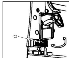
4. Make sure trigger and work contact element (WCE) move freely up and down without binding or sticking after each adjustment.
