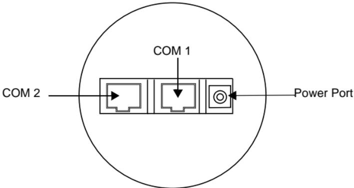
COM 1 connects to the host computer; COM 2 is used for daisy-chaining multiple cradles together; and, the Power Port supplies power to the cradle.
