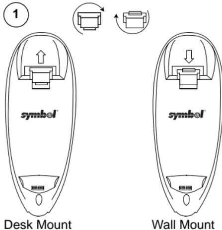
1. Lift the scanner support tab out of the top part of the cradle and replace it in the wall-mount position as shown.
