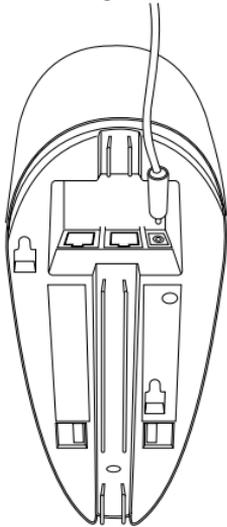
1. Insert the independent power plug into the Power Port. (The cradle cannot be powered by the host computer.)
