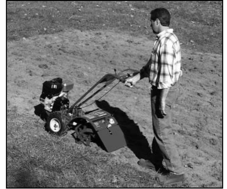
Figure 4-2: Use one hand to guide tiller when moving forward.
