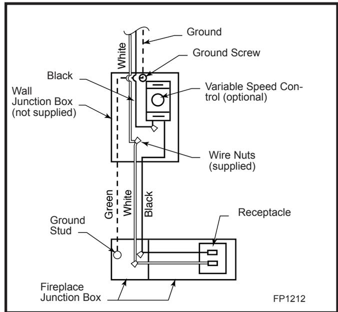
Fig. 9 SCVS wiring diagram.
