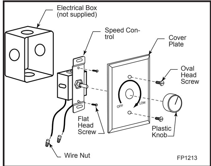
Fig. 10 Speed control mounting.
