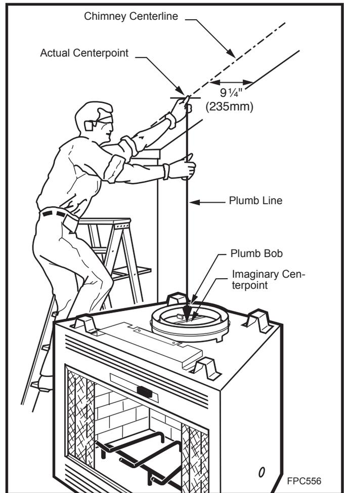
Fig. 11 Locate centerline of chimney with plumb line.
