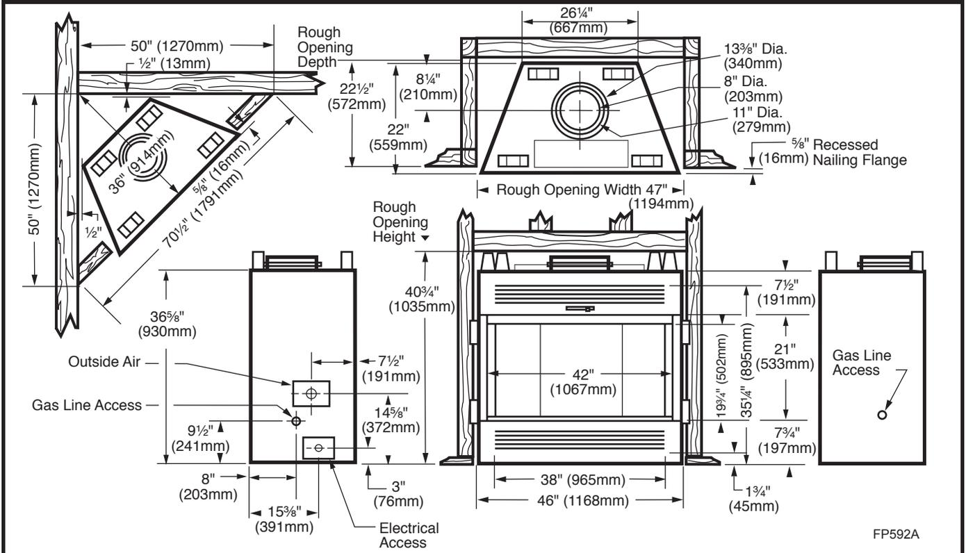
Fig. 2 WMC42 Series specifications and framing.
