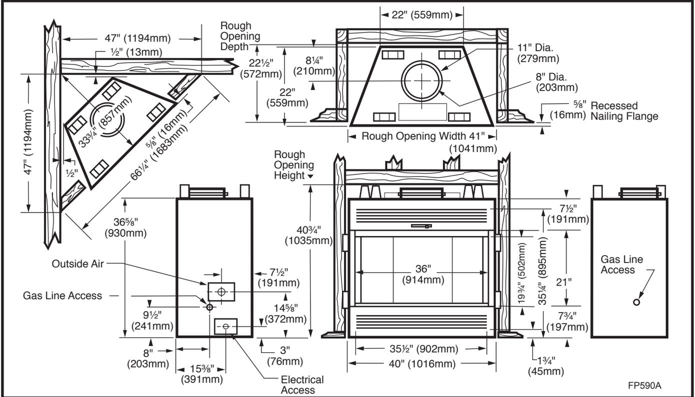
Fig. 1 WMC36 Series specifications and framing.
