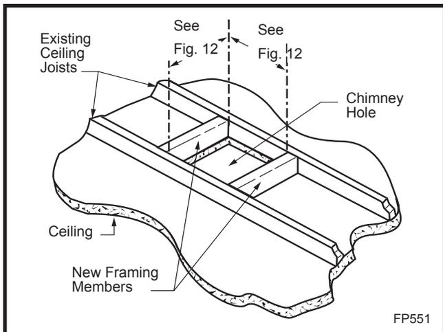
Fig. 13 Typical frame for ceiling chimney hole.
