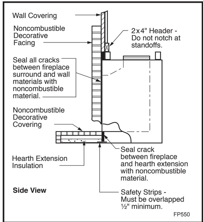
Fig. 26 Sealing gaps.
