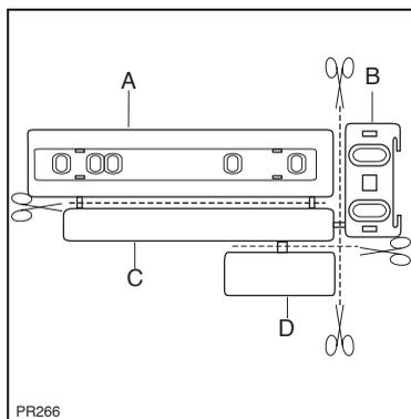
Place guide (A) on the inside part of the furniture door, up and down as shown in the figure and mark the position of external holes. After having drilled holes, fix the guide with the screws supplied.
