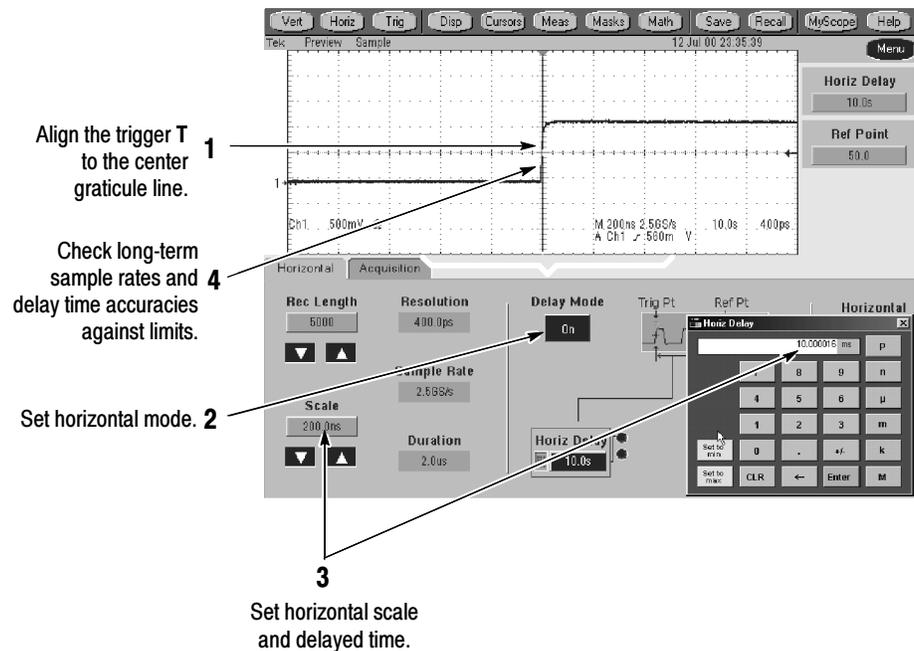
**Figure 2-17: Measurement of accuracy - long-term and delay time**
