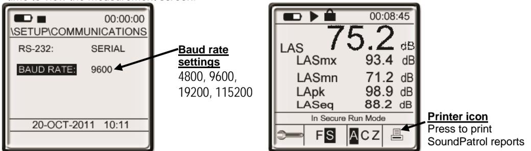
Figure 4-15: Baud rate setup and print icon
