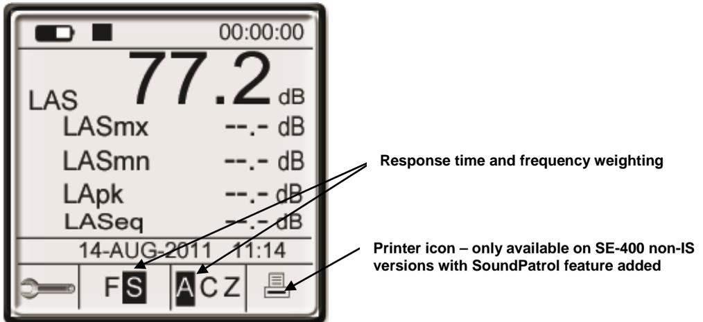
Figure 3-1: Response time and frequency weighting
