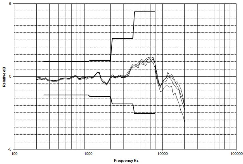
Directional frequency positioned side toward noise source ( $0^{\circ}$ - $90^{\circ}$  incidence angles)
