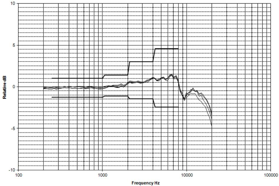
Directional frequency response positioned facing toward noise source ( $0^{\circ}$ - $90^{\circ}$  incidence angles)
