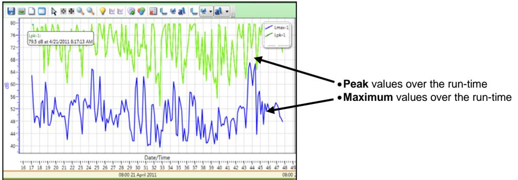
Figure 4-5: Example of logged data in DMS
