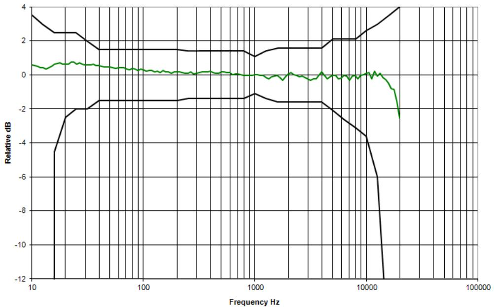
**Nominal BK4936 microphone frequency response, diffraction and reflection corrections (section: 5.2.8)**
