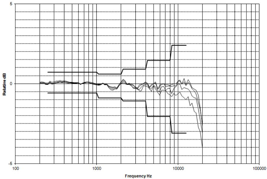
Directional frequency response positioned side toward noise source ( $0^{\circ}$ - $90^{\circ}$  incidence angles)
