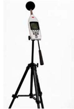
Figure 4-7: Measurement positioning and tripod mount
