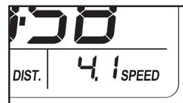
**The upper display**—The upper display can show the elapsed time, the distance that you have walked or run, the speed of the walking belt, or the approximate number of calories you have burned. Press the Priority Display button repeatedly until the upper display shows the information that you are most interested in viewing. Note: While information is shown in the upper display, the same information will not be shown in the lower displays.
