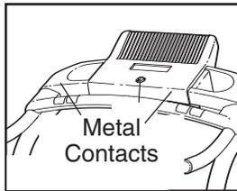
To measure your heart rate, **stand on the foot rails** and hold the metal contacts—**avoid moving your hands**. When your pulse is detected, the small heart symbol in the lower right display will flash, one or two dashes will appear, and then your heart rate will be shown. **For the most accurate heart rate reading, continue to hold the contacts for about 15 seconds.**
