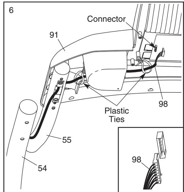
7. Insert the excess Wire Harness (98) down into the Right Upright (54). Then, tighten the two plastic ties around the Wire Harness, and cut off the ends of the plastic ties.
