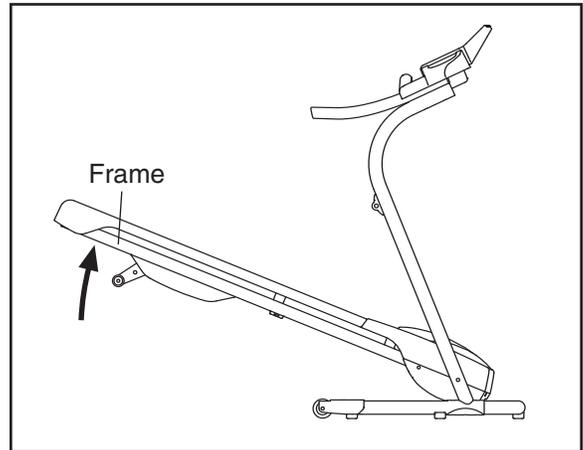
2. Move your right hand to the position shown and hold the treadmill firmly. Using your left hand, pull the latch knob to the left and hold it. Raise the frame until the catch is past the latch pin. Then, slowly release the latch knob; make sure that the latch pin is resting against the catch.
