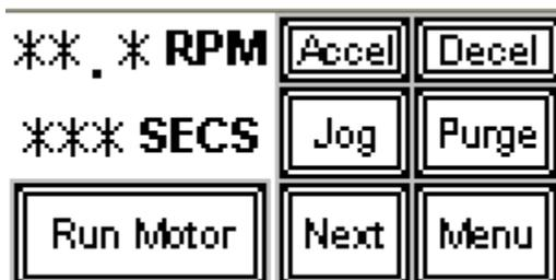
This screen is only available when the A250 control is stopped. This screen provides the means to purge / clear additive, prime additive, etc..
