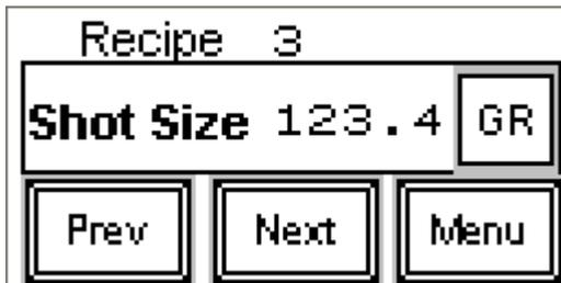
The shot size specifies the total capacity of the mold in use on the press. The value can be entered in grams, kilograms, ounces, or pounds. The unit of measure is changed by pressing the units button at the middle right of the screen. Changing the unit of measure will NOT change the value displayed on the screen.
