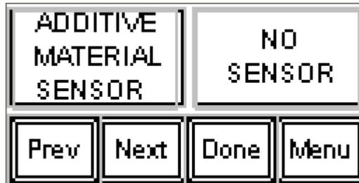
**Additive sensor.** Select the no sensor, alarm only, or alarm & stop.
