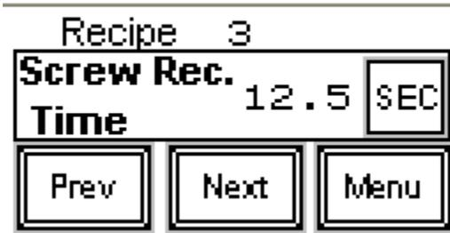
The screw recovery time is the estimated screw recovery time, and is used as the initial value for validating the recipe. Actual screw recovery times as measured by the presence of the screw recovery signal, are used to fine-tune the feed rate during operation. The estimated time **must** be at least ½ of the actual recovery time. If less than ½, the feeder will interpret the recovery signal as a purge cycle.
