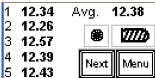
Displays the 5 most recent screw recovery times (latest on top), as well as the simple average and weighted average.
