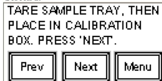
Initial preparation for weighing samples. The access cover to the calibration chamber should be removed / opened. The container used to catch and hold the samples should be tared (place the container on the scale and zero the scale). The container should then be placed in the calibration chamber. Press “Next” when these steps have been completed. The motor will begin to run as Screen 2 will be displayed.
