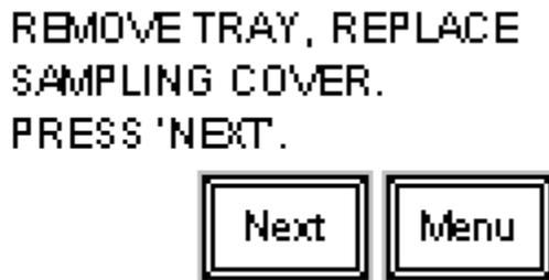
The tray should be removed from the calibration chamber. The access cover should be replaced / closed. Weight Calibration is complete. Note that at any time in the process, the “Menu” button may be pressed to abort the weight calibration process. Any sample weights, if any, are used to calculate the average weight. If no sample weights are entered, the calibration weight is used for calculations. Using less than 5 samples may affect feeder accuracy.
