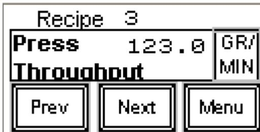
Press throughput specifies the total weight of material through the extruder per minute. The value can be entered in grams, kilograms, ounces, or pounds per minute. The unit of measure is changed by pressing the units button at the middle right of the screen. Changing the unit of measure will NOT change the value displayed on the screen. It is important that this value be adjusted whenever the extruder speed changes.
