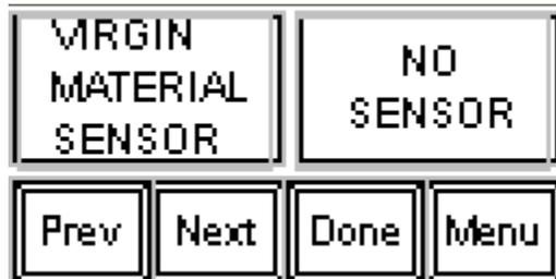
**Virgin material sensor.** Select the no sensor, alarm only, or alarm & stop.
