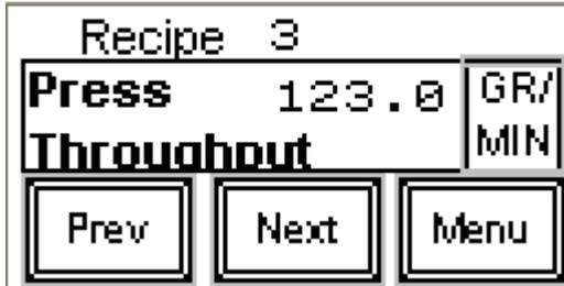
Press throughput specifies the total weight of material through the extruder per minute. The value can be entered in grams, kilograms, ounces, or pounds per minute. The unit of measure is changed by pressing the units button at the middle right of the screen. Changing the unit of measure will NOT change the value displayed on the screen. It is important that this value be adjusted whenever the extruder speed changes.
