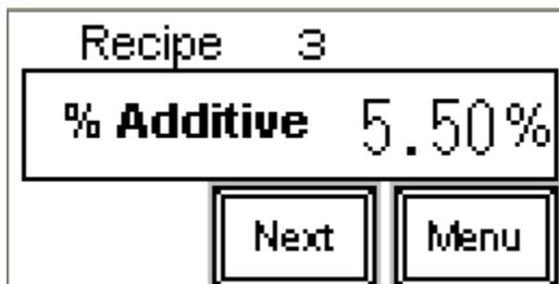
The % additive specifies the proportion of additive to virgin material as a percentage of throughput. For example, if the throughput is 200 grams per minute and 8.5 grams of additive are required, the additive percentage would be 4.25. After the additive value has been entered, press the “Next” button to navigate to the Throughput screen.
