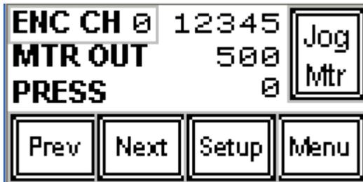
This screen monitors the analog input & output, as well as the raw encoder value input. Additionally, the encoder can be connected to an alternate PLC input to help troubleshoot encoder problems. To change the encoder input, disconnect power & move the encoder signal wire from input 0 to any of inputs 1, 2, or 3. Restore power, navigate back to this screen, and change the “ENC CH” # to match the PLC input chosen.
