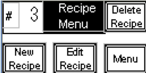
The Recipe menu allows selection, editing, and deletion of recipes. The current recipe is displayed in the upper left corner. A different recipe can be selected by pressing the recipe value. Selecting a new recipe will automatically change the screen to the 1<sup>st</sup> recipe entry/editing screen.
