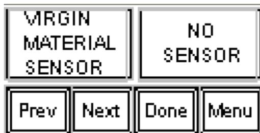
Virgin material sensor. Select the no sensor, alarm only, or alarm & stop.
