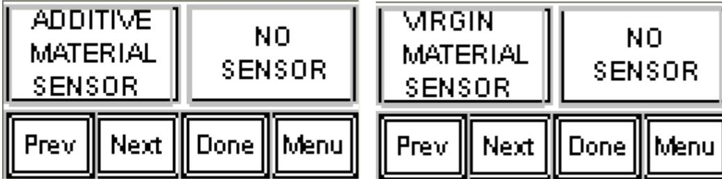
These screens select whether an additive (or virgin) material sensor is present and if so, what action to take when the sensor detects no material. Press the button in the upper right corner to sequence through the following options:
