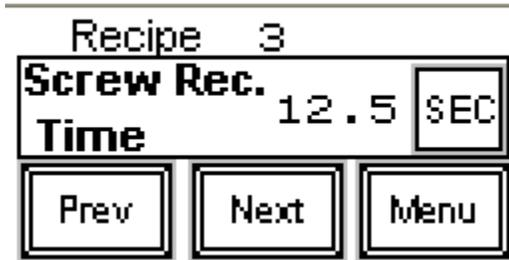
The screw recovery time is the estimated screw recovery time, and is used as the initial value for validating the recipe. Actual screw recovery times as measured by the presence of the screw recovery signal, are used to fine-tune the feed rate during operation. The estimated time **must** be at least  $\frac{1}{2}$  of the actual recovery time. If less than  $\frac{1}{2}$ , the feeder will interpret the recovery signal as a purge cycle.
