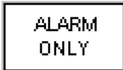
Sensor is present. Display alarm screen & activate alarm output, but keep feeder running.
