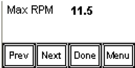
The maximum motor RPM is the maximum rated speed for the motor being used with the A250 control. The default nominal value is 11.5 RPM. This value should be changed to reflect the actual motor RPM based on motor type and tuning results (See **Drive Tuning** following this section). Initially, this value should be set to the nameplate RPM for the motor/gearbox being used, before proceeding to Drive Tuning.
