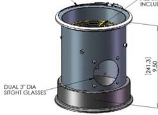
892.01982.00 - 4.4L SUPPLY HOPPER, DD/DP DP UNIT REQUIRES 2 ROLL PINS(CT144027)
