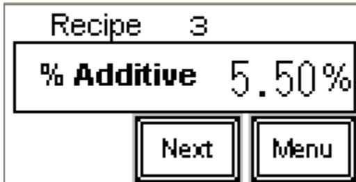
The % additive specifies the proportion of additive to virgin material as a percentage of throughput. For example, if the shot size is 200 grams and 8.5 grams of additive are required, the additive percentage would be 4.25. After the additive value has been entered, press the “Next” button to navigate to the Shot Size screen.
