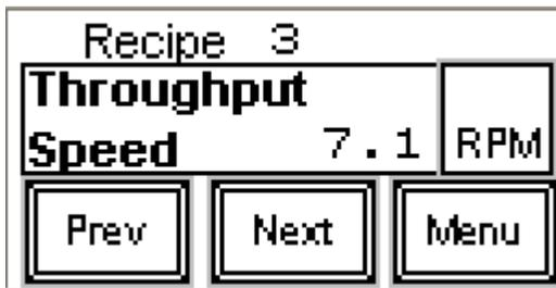
The press speed corresponding to the throughput value entered on the previous screen. Given these reference values, the correct feed rate can be determined for any extruder speed. Note that the minimum and maximum press speeds and signal levels must be entered correctly in Setup.
