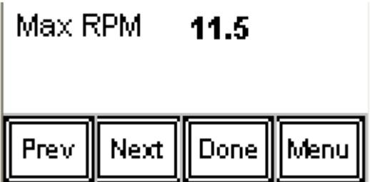
**Maximum Motor speed.** Enter nominal motor speed.
