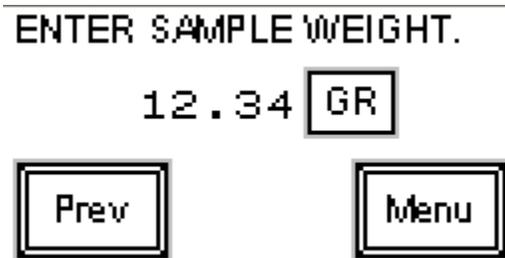
Enter the sample weight obtained from the previous cycle of the feeder. The unit of measure will be the same as used for the calibration weight. Pressing the Enter symbol on the screen keypad displays Screen 7.
