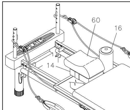
Make sure that both **FOAM PADS(16)** are in the carriage when using the **HEADPAD(60)** attached to the **HEADREST(14)**.
