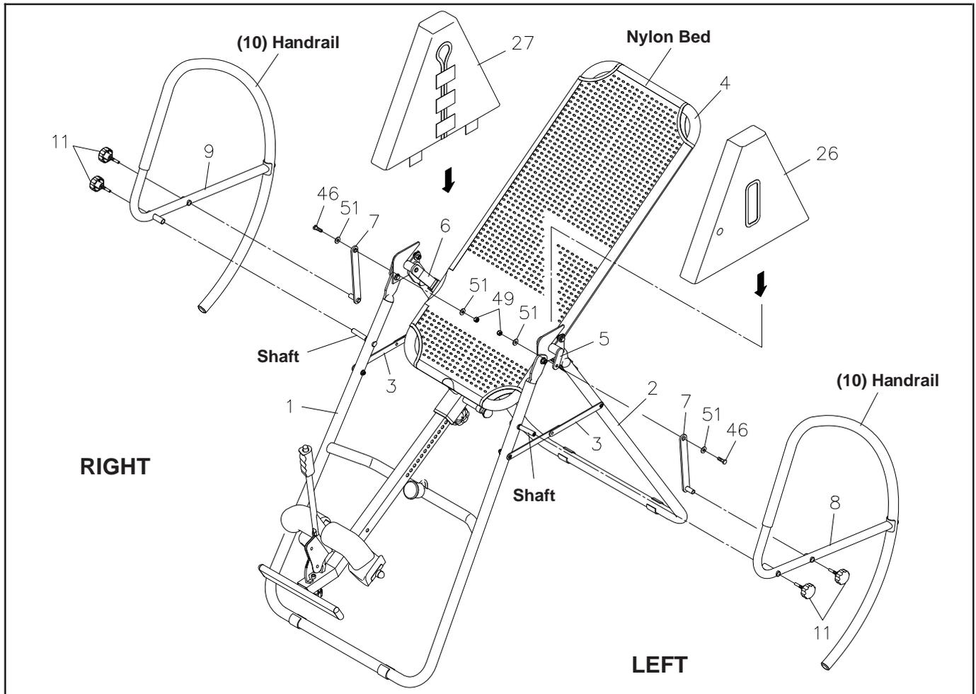
**STEP 10:** Slide the **LEFT** and **RIGHT PROTECTIVE COVERS(26, 27)** onto each side of the **BASE ASSEMBLY**. Make sure the **SHAFTS** on the **FRONT FRAME(1)** poke out through the hole on the **PROTECTIVE COVERS(26, 27)**.
