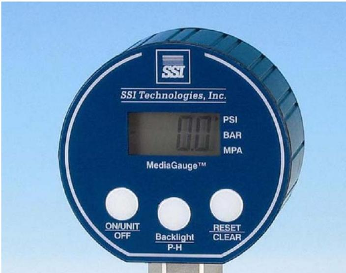
The *ON/UNIT/OFF* button is used to display the pressure reading; switch between pressure units (PSI; BAR; and MPA) and to power down the unit.
