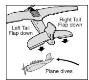
Gently bend both HORIZONTAL TAIL FLAPS down to prevent plane from crashing/stalling.
