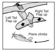
Gently bend both HORIZONTAL TAIL FLAPS up to make the plane **climb higher/faster**.
