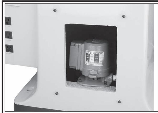
**Figure 57. Location of coolant pump.**
