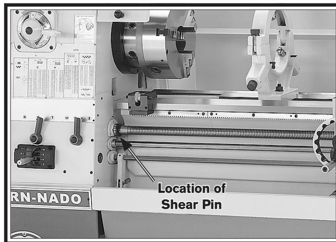
**Figure 132. Location of shear pin.**
