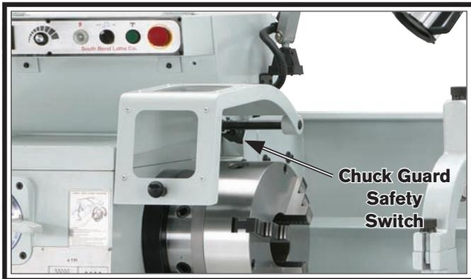
Figure 151. Chuck guard limit switch.
