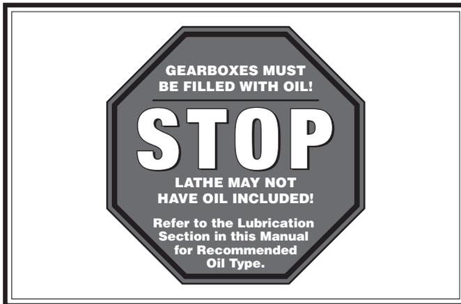
The headstock, quick-change gearbox, and apron oil reservoirs must have the proper amount of oil in them before the lathe can be operated for the first time.
