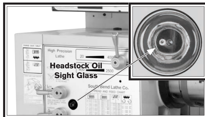
Figure 109. Location of the headstock oil sight glass.
